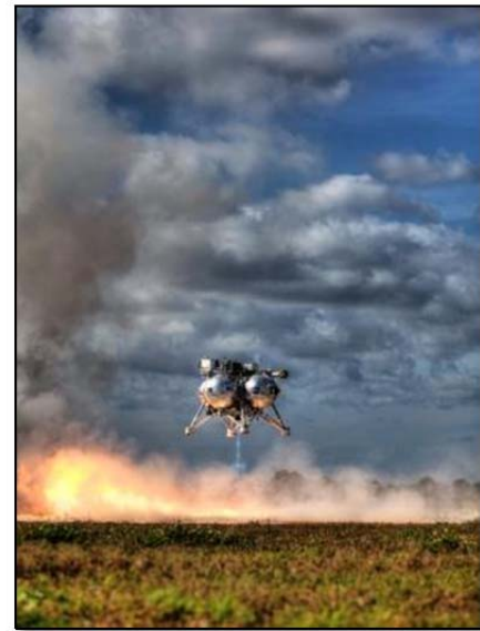
Morpheus liftoff over a flame trench at the KSC SLF
