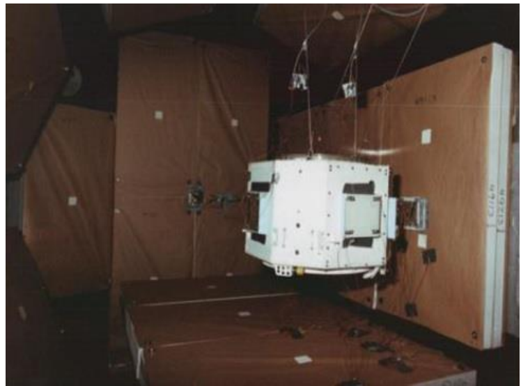
Fig 1. SOCIT Test Article with Multilayer Foam Soft Catch
