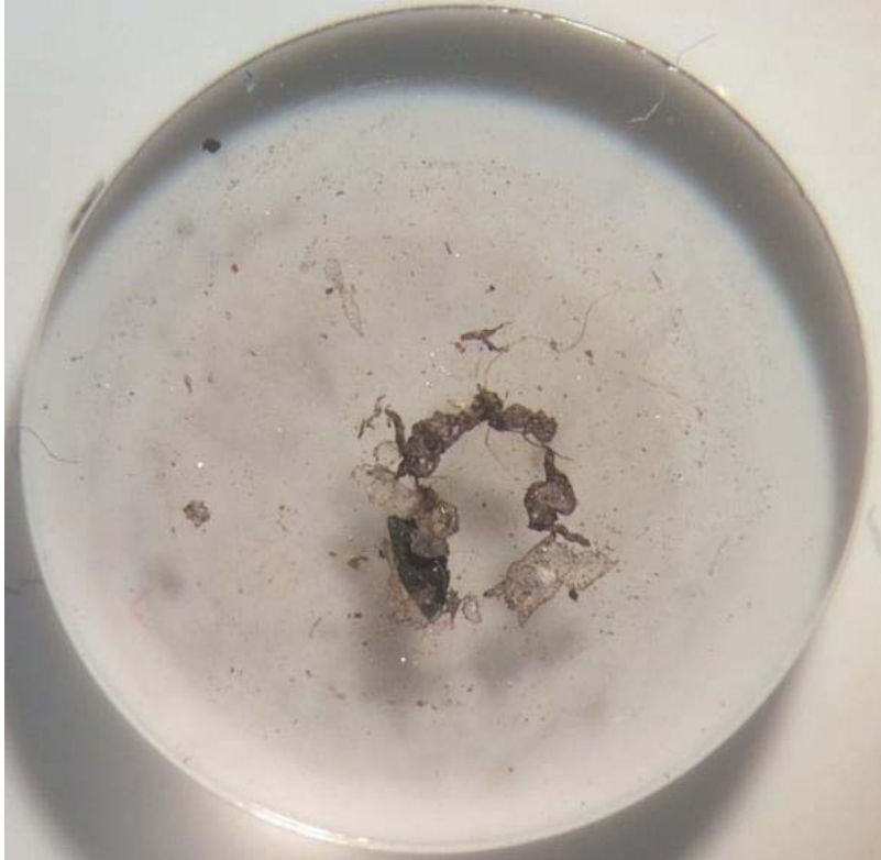
Figure 6. Material deposited on bottom sapphire window
