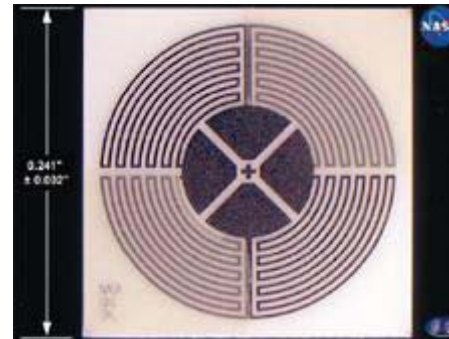
Heat Flux Sensor Array to T=1000°C
