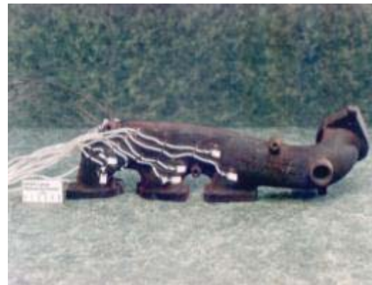
1991 R&D 100 Award PdCr wire strain gauge applied on Ford Motor Co. exhaust manifold Glenn Research Center
