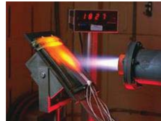
1998 R&D 100 Award Long-lived Convoluted Thermocouples For Ceramic Temperature Measurements
