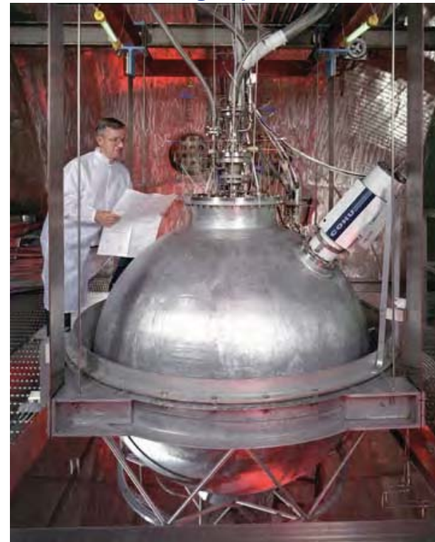
1990s - Liquid hydrogen tank in test at the Cryogenic Propellant Tank Facility (K-Site): fill, pressurization/venting, slosh
