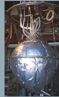
LH2 Zero Boil-off storage feasibility demonstrated (1998)
