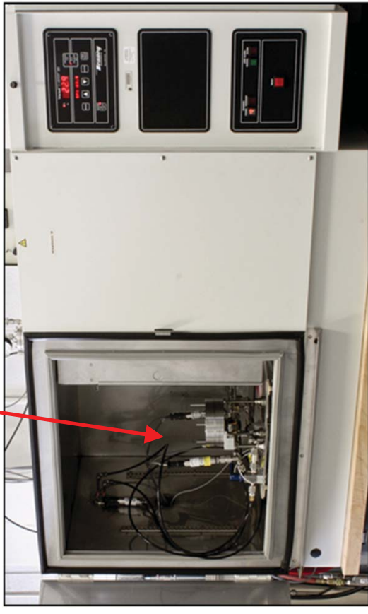
Test fixture inside environmental control chamber
