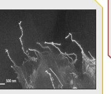
Creating nanomaterial with unique structure could effectively improve the lithium storage properties of the metal oxide. The SEM shows that a unique approach is developed to attach  $Fe_2O_3$ uniformly on CNTs.
