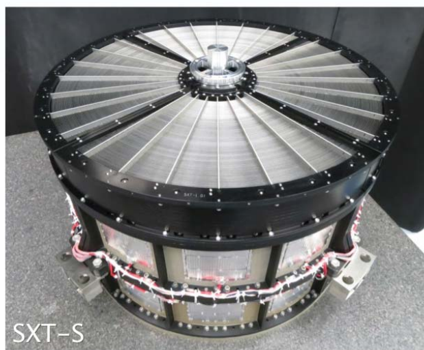
Astro-H has two identical Soft X-ray Telescopes, SXT-I and SXT-S. Both mirrors exceed their requirements for collecting area and imaging performance.
