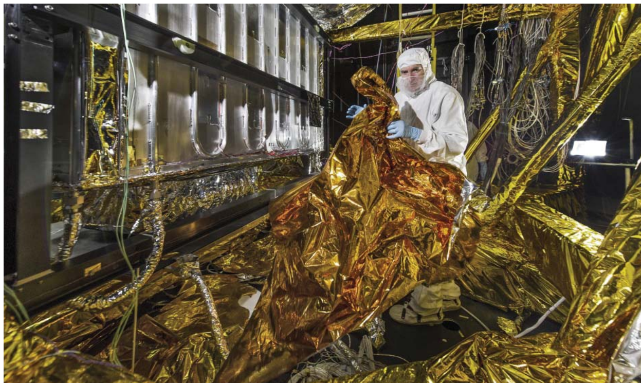
Goddard engineer Ed Shade puts the final touches on thermal blankets in a Space Environment Simulator, a vacuum chamber used to test JWST components. The blankets, made of aluminized kapton, cover wiring on the floor to prevent the heat they create from contaminating the other parts of the test bed. Credit: NASA/Chris Gunn
