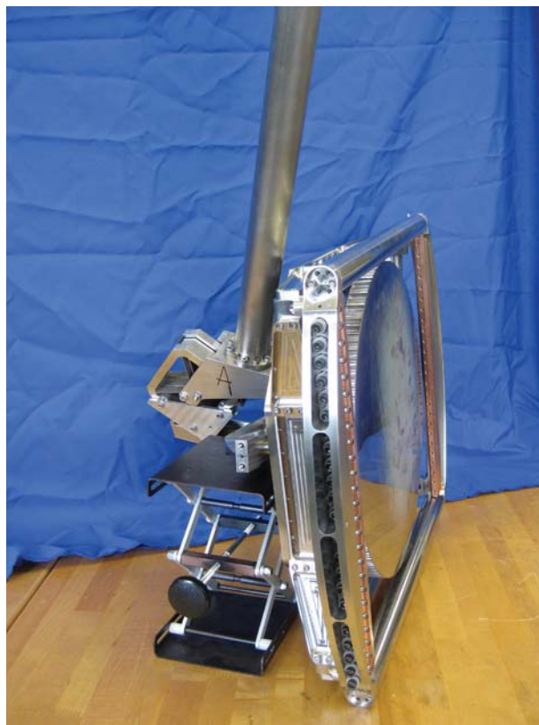
The PIPER Variable-Delay Polarization Modulator. The polarizer uses 1.5 km of 36 \mu\text{m} diameter wire, held to 3-micron precision across a 40-cm aperture. The VPM operates at 1.5 K using simple linear translation of the reflective mirror.
