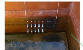
Alternating Seawater Spray Test:
