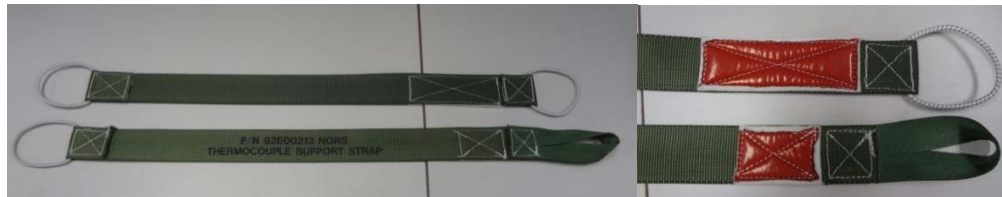
Figure 3 - Comparison of the new and old RTA straps (Top and bottom respectively)
