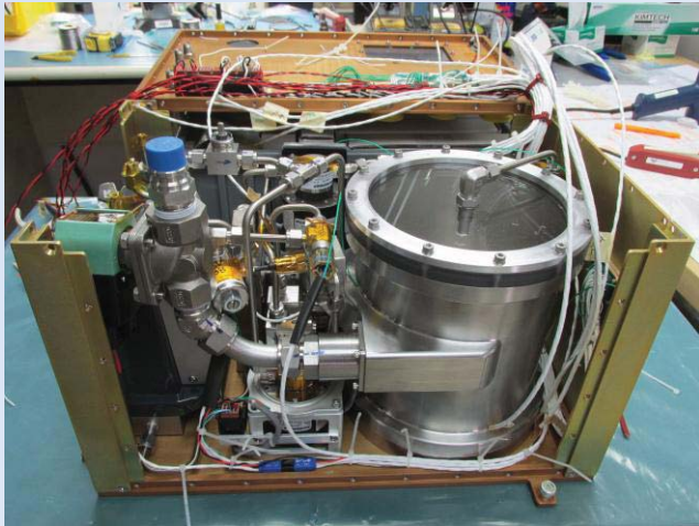
Pumped Separator for PBRE
