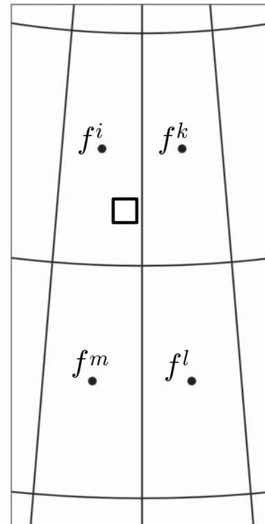
**Fig. 8.** Setup for bilinear interpolation. The value in an ice grid cell (square) will be the sum of the values at the four nearest atmosphere grid cell centers, weighted by  $\Delta$ -longitude and  $\Delta$ -latitude along the axes.
