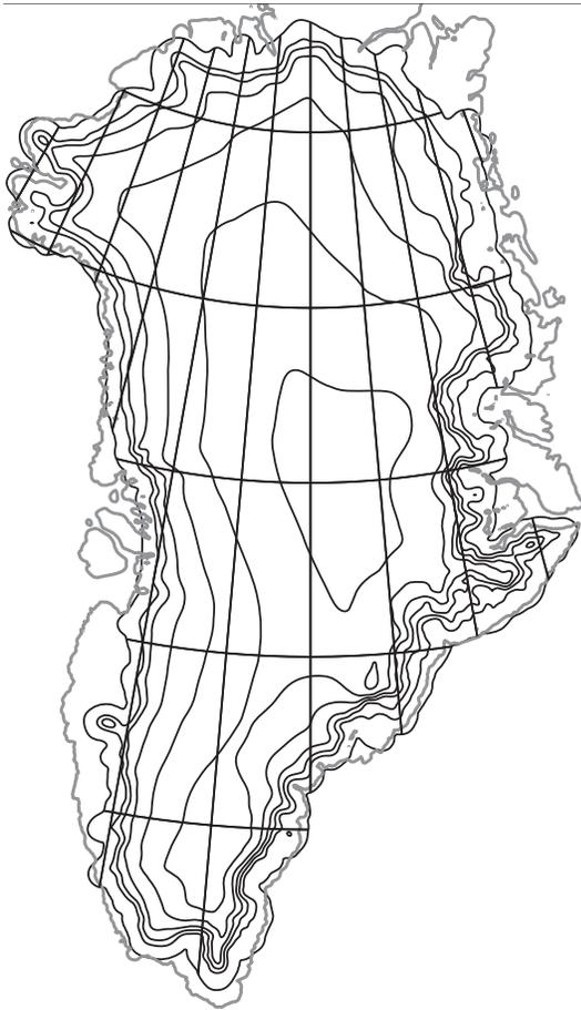
**Fig. 9.** Traditional elevation class schemes are equivalent to running the ice surface model on an L0 grid, where grid cell outlines are created by the intersection of the atmosphere grid and elevation contours. One such grid is shown in this figure. Note that grid cells extend only as far as the ice sheet; the grey line shows the Greenland coast.
