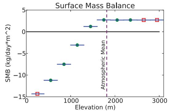
**Fig. 10.** Interpolated SMB function within one atmosphere grid cell when using elevation classes. The resulting piecewise constant interpolation is almost never preferable to the piecewise linear interpolation in Fig. 4. Traditional elevation class schemes are discouraged because they offer no benefit over first-order  $z$  interpolation.
