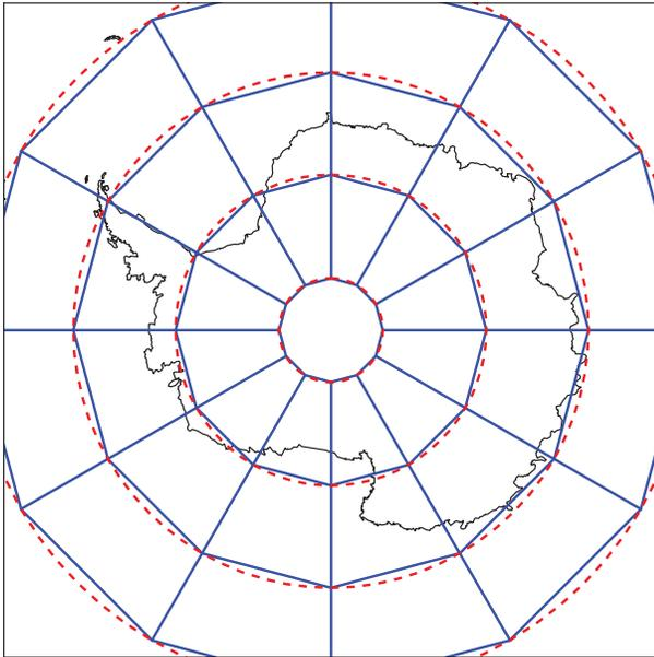
**Fig. 6.** An example of geometric error, in which grid cells change size due to polygonal approximation. This map, made using a Lambert equal area projection centered on the North Pole, shows a set of latitude–longitude grid cells – a kind commonly used in atmosphere models. Solid blue lines show polygonal approximations, while dotted red shows the actual grid cells on the sphere. Note that all grid cells (in this local map) shrink when approximated.
