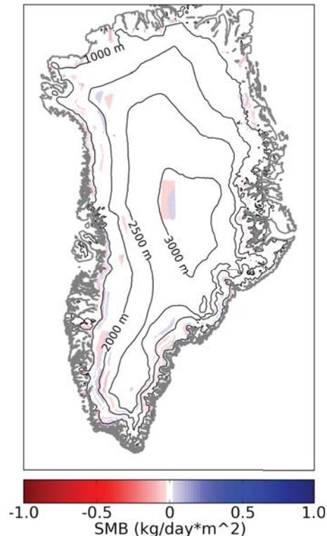
**Fig. 16.** Example of numerical dispersion caused by an ill-posed quadratic optimization problem. July SMB on elevation grid  $E$  was regridded to the exchange grid. The reverse transformation was then used to recover the original SMB on  $E$ . Plot shows the difference between the result and the original. In theory, the two should be exactly the same. Although mass is conserved, differences appear because the associated quadratic optimization problem is underdetermined in some areas.
