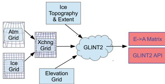
**Fig. 21.** The Glint2 workflow used to compute the regridding operations required by the fully coupled system (Fig. 2). Glint2 produces regridding operations based on a variety of factors: atmosphere and ice grid geometry, ice topography and extent, and levels chosen for the elevation grid. Glint2 must recompute the operations when any of these factors changes.
