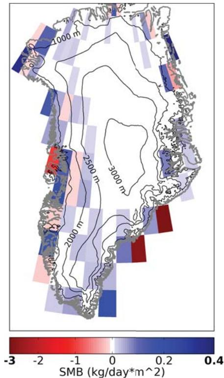
**Fig. 15.** Difference in July SMB obtained with  $E \rightarrow A$ , using two choices for the interpolation grid  $G$ : either the exchange grid or the ice grid. Differences (exchange minus ice) are due to ice grid cells that overlap more than one atmosphere grid cell.
