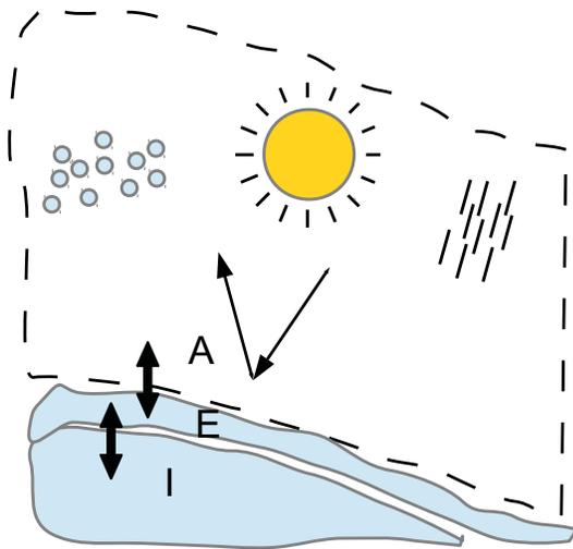
**Fig. 1.** Configuration of the three models, and the separate spatial domains they occupy. The atmosphere model (*A*) is coupled to the ice surface model (*E*), which tracks the top few meters of ice. The ice surface model (*E*) is then coupled to the dynamic ice flow model (*I*). The dynamic ice flow model, operating at long time steps, is insulated from high-frequency surface processes in the ice–atmosphere interaction.
