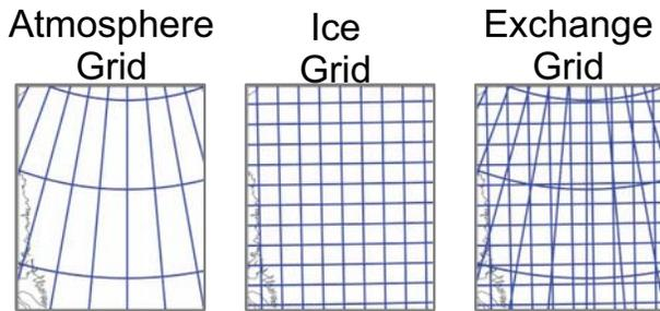
**Fig. 5.** An exchange grid, obtained by overlapping a sample atmosphere grid and ice grid (not to scale). Each resulting grid cell, irregularly shaped, overlaps with exactly one atmosphere grid cell and exactly one ice grid cell.
