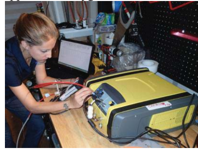
Fig. 6: Crew member taking samples in the shipping container using the portable Gasetm FTIR.
