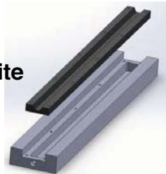
Above: Test Piece highlighting ZrC Coating Right: Coating primarily on external surface
