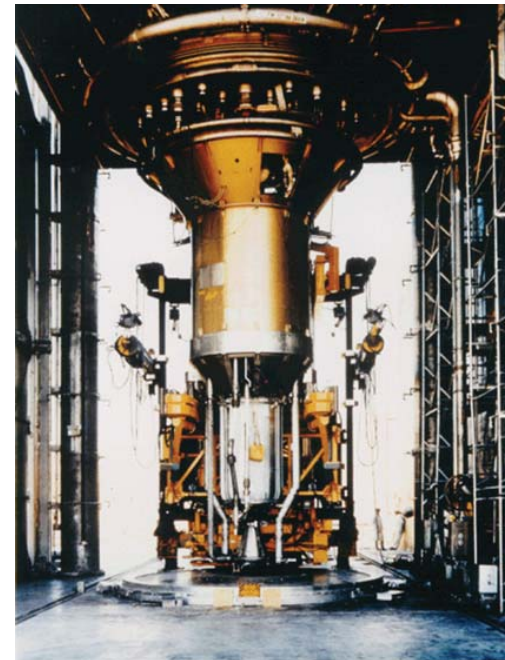
The NERVA Experimental Engine (XE) demonstrated 28 start-up / shut-down cycles during tests in 1969.
