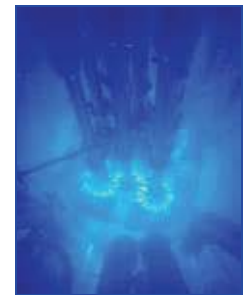
Fuel Element Irradiation Testing in ATR at INL
