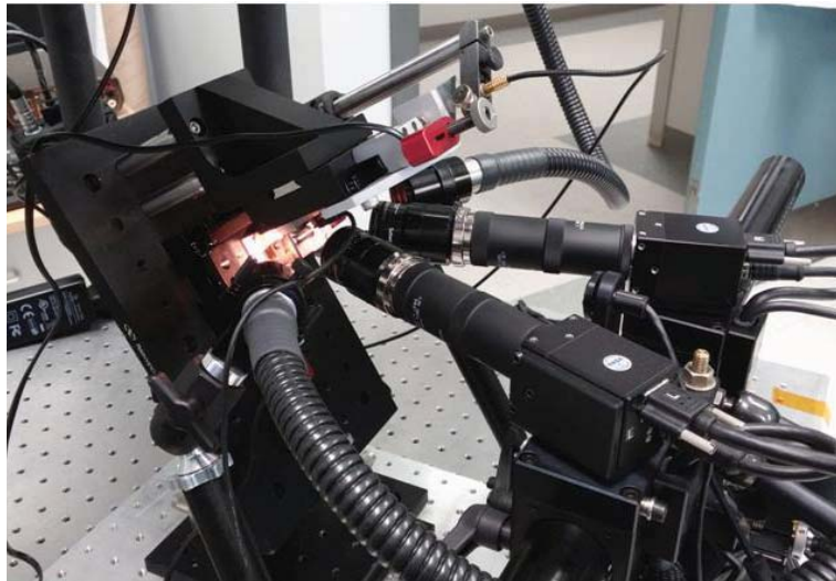
Figure 3. Setup for the verification of the capacitive displacement gauge using dual camera (stereo) DIC system (microAramis). Using this system, the position of a surface point very close to the probe tip could be tracked in 3D space.
