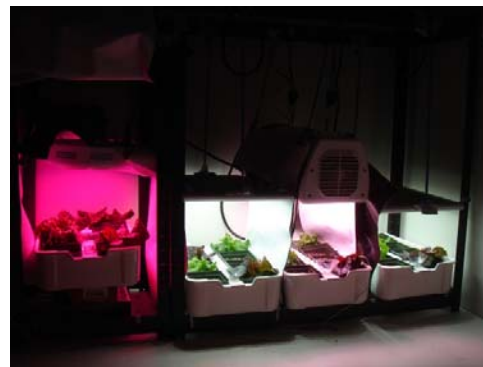
Fig. 4: Lamp set-up in the sciences lab. Left to right: red and blue UFO LED lamp, KSC white panel, Heliospectra LX 60, and KSC white panel.
