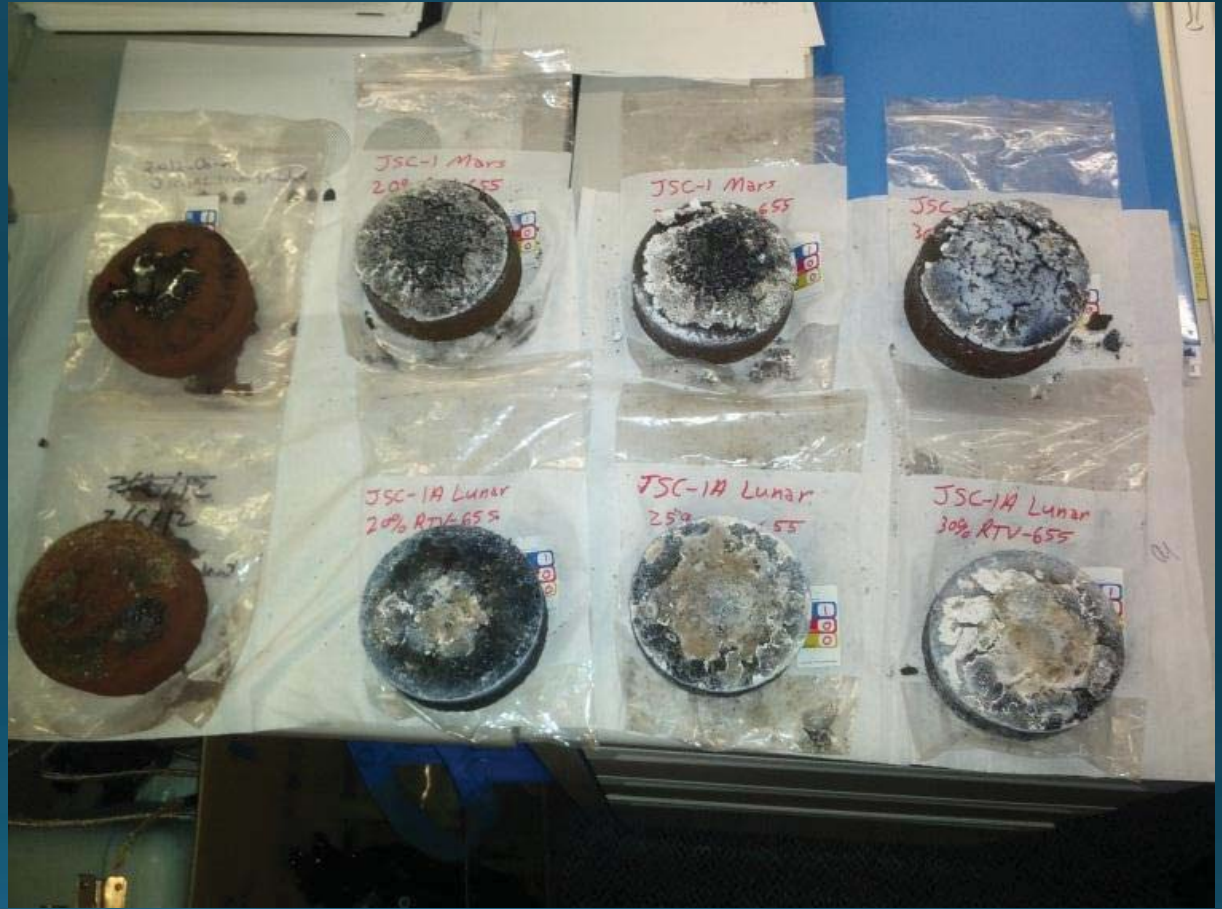
Clockwise from top left: Regolith-derived heat shield sample undergoing flame testing; regolith samples post-test; artist concept. Image Credit: NASA/KSC
