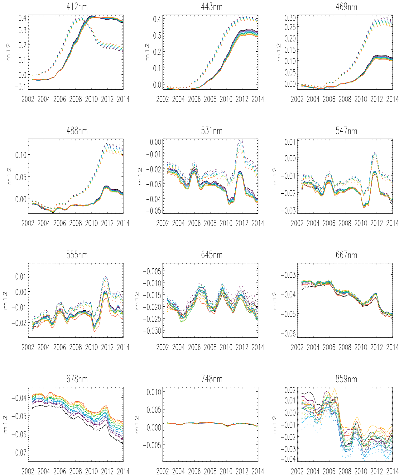
Figure 10. m_{12} for mirror sides 1 (solid line) and 2 (dashed line), detectors 1-10 (black to red) of MODIS Terra as a function of time for all wavelengths at the end of scan scan (frame 1250).
