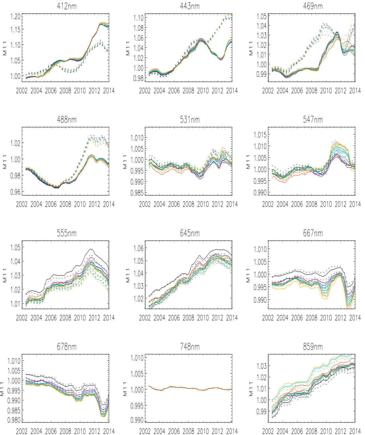
Figure 9. M_{11} for mirror sides 1 (solid line) and 2 (dashed line), detectors 1-10 (black to red) of MODIS Terra as a function of time for all wavelengths at the end of scan scan (frame 1250).
