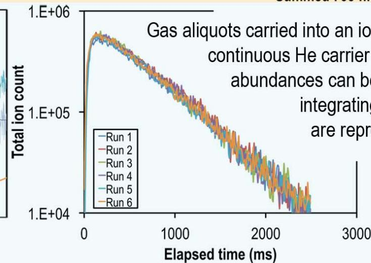
Gas aliquots carried into an ion trap MS by a continuous He carrier flow show that abundances can be measured by integrating over time and are reproducible to 3%.
