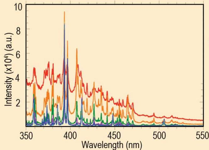
LIBS spectra are collected with every shot or gated over multiple shots (left). Spectra are corrected for background, normalized to total radiance, and continuum subtracted before [K] is determined by peak areas referenced to standards (right).
