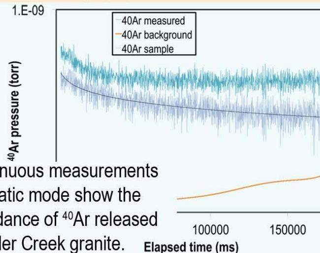
QMS continuous measurements made in static mode show the total abundance of  $^{40}\text{Ar}$  released from Boulder Creek granite.
