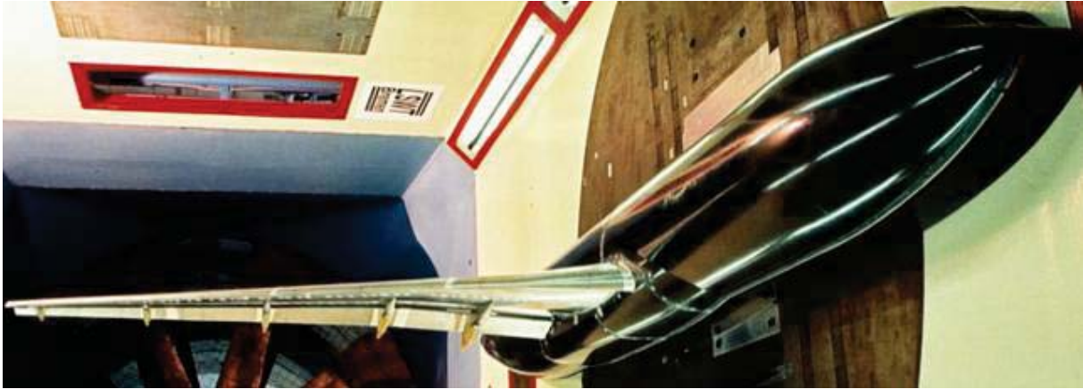
Figure 1. DLR-F11 high-lift wind tunnel model in the Airbus Low Speed Tunnel in Bremen (B-LSWT).
