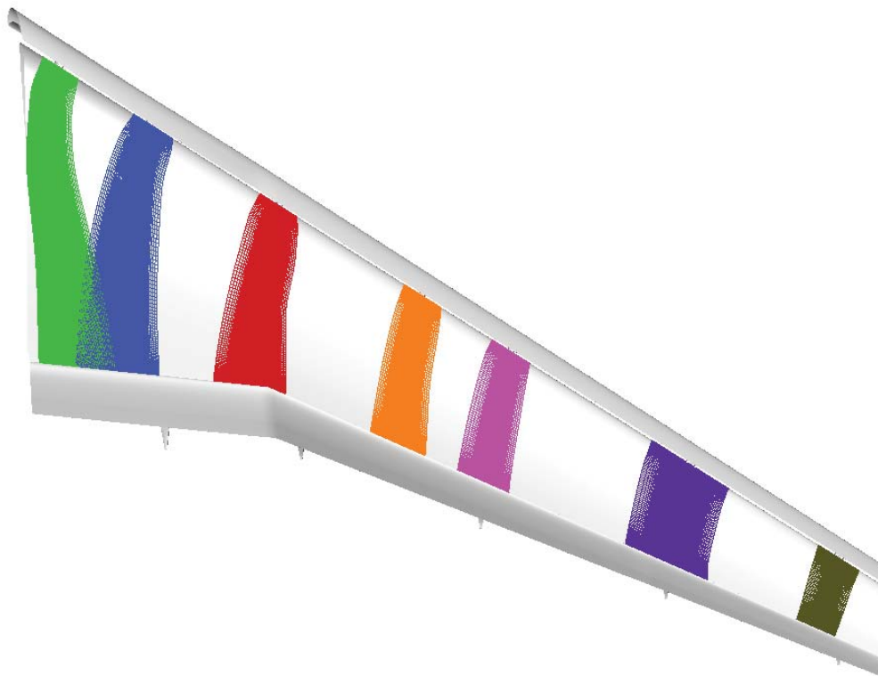
Figure 33. Wing planform view showing surface grid planes of PTB patch grids with increased size/density behind bracket 6 (purple grid).
