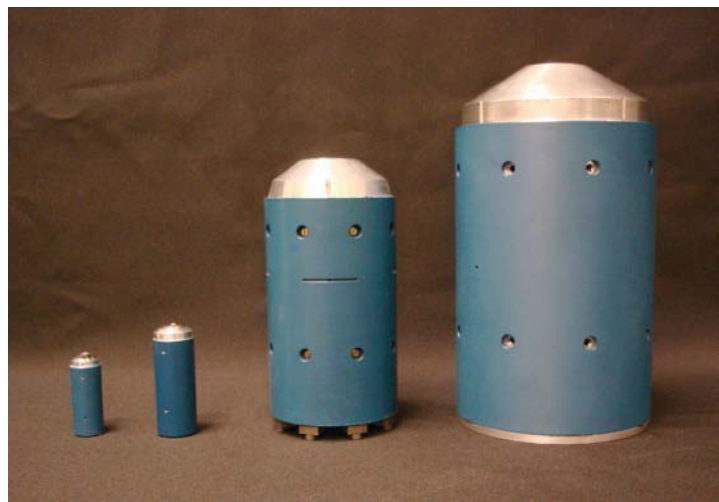
Figure 10. Scaled ASC technology - Pistons from existing Sunpower convertors, left-to-right: 35 W SBIR, 80 W ASC, 1 kW convertor, and 6kW piston (two used for the 12 kW PCU)
