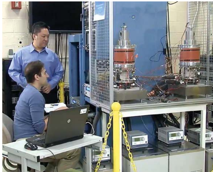
Figure 6. ASC-E3 Pair 1 (#1 & #2) in individual Common Performance Hardware under vertical performance testing at GRC's SRL
