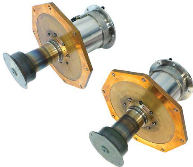
Figure 8. Completed Flight-like ASC-E3 Pair 3 Convertors
