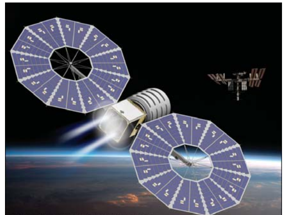
Figure 1. L2 Logistics Support Mission. Spacecraft capable of delivering 5000 kg payload to EM-L2.
