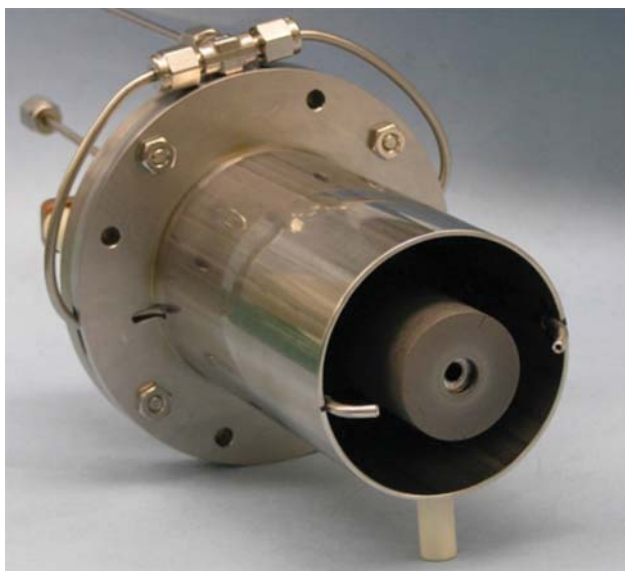
Figure 2. The JPL-developed \text{LaB}_6 cathode assembly, complete with the cathode plume external gas injectors. Reproduced from figure 4 in Ref. 17.
