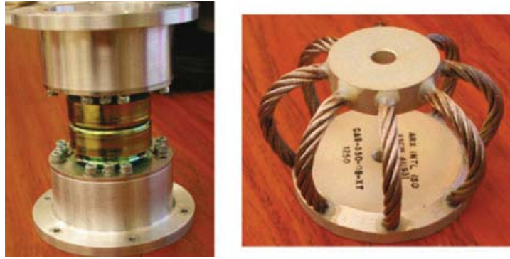
Fig. 6 Rubber dampers from Barry Control with attachment fixtures ( left ) and wire rope isolator from Isotech, Inc. ( right ). The wire rope isolators are shown suspending the cryostat in Fig. 2. (Color figure online)
