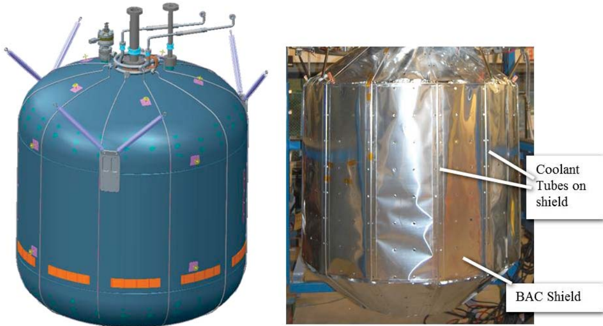
Figure 4. Tube-on-tank on left, tube-on-shield concept on right.
