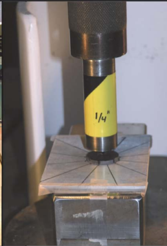
Ball on disk set-up
