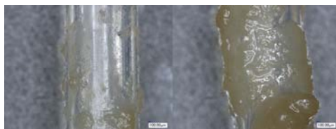
Figure 6: Biofilms present on samples after fiber harvest for TTU inoculum with control (Left) fibers and FE 18-sec-treated (Right) fibers showing drastic cell attachment differences.
