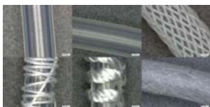
Figure 1: Various fiber treatments tested: Top: PE (5 sec), 1500-Grit Sanding, Cable Sheath Bottom: Cotton thread, Silk Thread, Spider Silk
