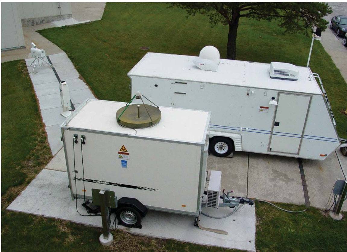
Figure 2.—NIRSS hardware. METEK Ka-band radar in foreground, Vaisala ceilometer in middle left, and Radiometrics MP3000 in back left.
