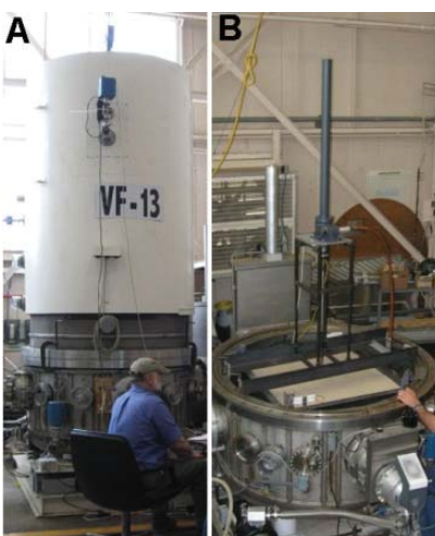
Figure 1.—Photo of the vacuum facility (A) with the lid and (B) without the lid, showing the research hardware. The tall structure is the cone penetrometer.
