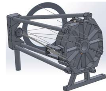
Prototype telescope spacer demonstrates dimensional stability and for studying scattered/stray light
