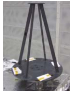
Prototype telescope spacer demonstrates dimensional stability and for studying scattered/stray light
