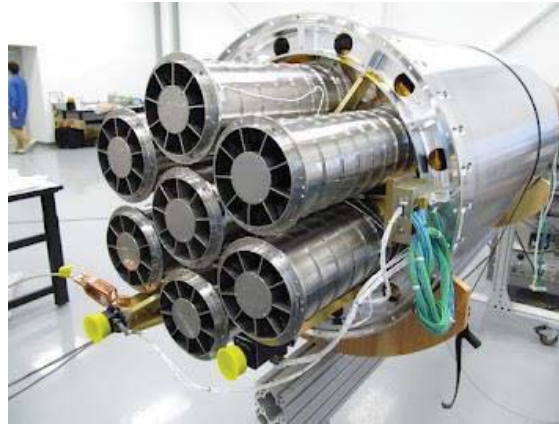
Replicated optics telescope modules (7 shells & 7 mod
