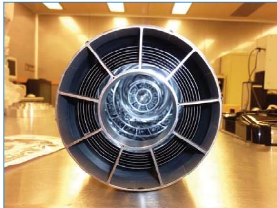
Replicated optics telescope modules (7 shells & 7 mod
