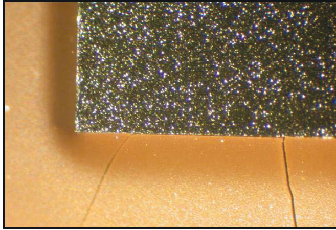
Figure 3-4. Underfill breakdown at the edge of a die with the longer underfill fillet.
