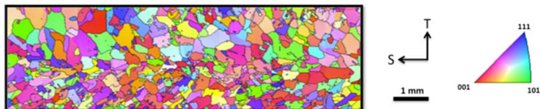
Figure 4. L-axis inverse pole figure map in IN 718 EBF 3 block (HT condition).
