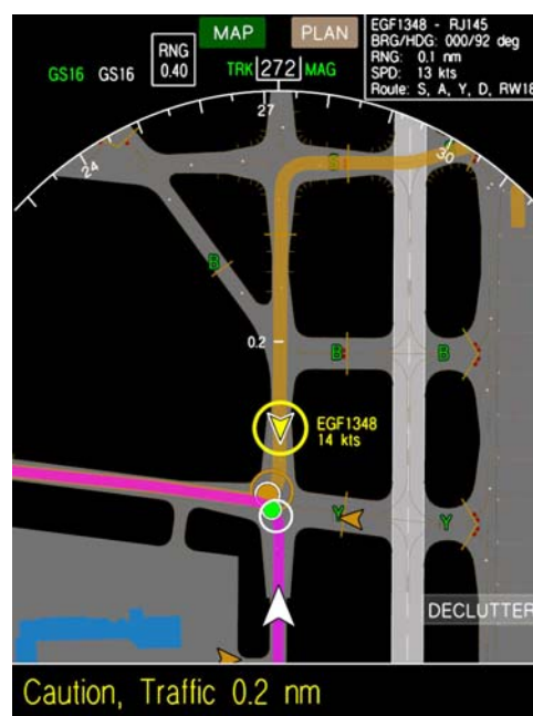
Figure 2. AMM Showing Caution Alert
