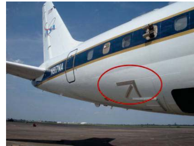
Figure 18. Adhesive tape testing holding wire samples in three polarizations (circled).
