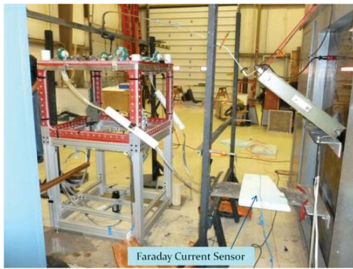
Figure 8. A high-current measurement setup.
