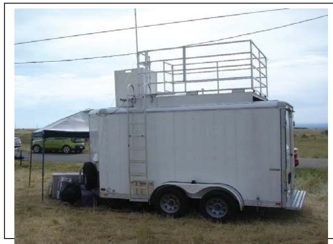
Fig. 4 Ozone lidar trailer at Table Mountain, Golden, CO.
