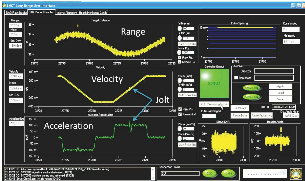
Figure 4. The coherent lidar system user interface illustrating track information. The lidar algorithm provides real-time range, velocity, and acceleration tracks as well as a number of other diagnostic signals. Note its ability to see acceleration jolts at the target turn-around points.
