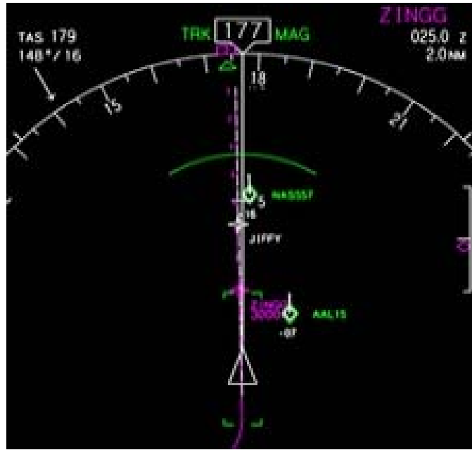
Figure 22. ND with “conformance box” during IMSPiDR.
