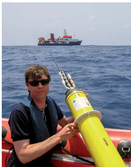
Figure 1 | Ocean observations. Martin Visbeck deploying an Argo float in the ocean from the research vessel MV Maria S. Merian . Argo is an international network of more than 3,000 robotic floats that measure the temperature and salinity of the ocean's upper 2,000 m.
