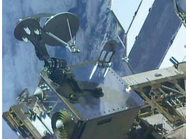
Figure 1.—SCaN Testbed Installed on ISS.
