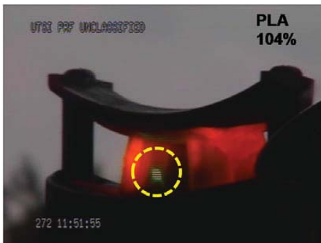
Figure 8.—Front view of Cr:GAP-coated Honeywell stator vane doublet in afterburner flame of J85 test engine at UTSI.
