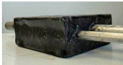
Figure 28.—Advanced thermal management concepts (Refs. 47 to 49). Graphite foam photograph reprinted from Carbon, vol. 41, Gallego, Nidia C.; and Klett, James W., Carbon Foams for Thermal Management, pp. 1461–1466. Copyright 2003, with permission from Elsevier.
