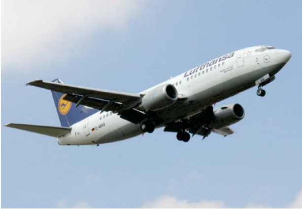
Figure 3.—Boeing 737-300—an example of a 150-passenger aircraft (Ref. 4). Arpingstone grants anyone the right to use this work for any purpose, without any conditions, unless such conditions are required by law.
