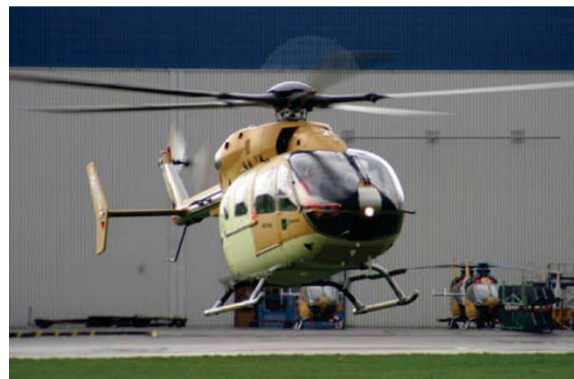
Figure 33.—Eurocopter equipped with bearingless rotor hub (Ref. 71). © Eurocopter, now Airbus Helicopters; used with permission.
