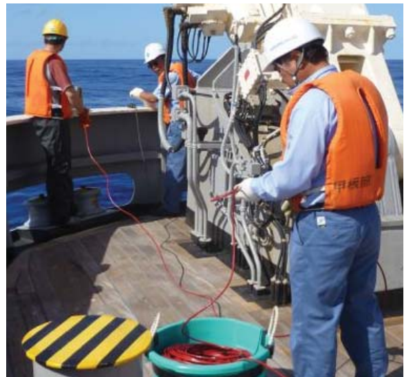
Fig. 21. A fair lead between the cable bucket and the point where C-OPS is being deployed over the stern of the R/V Hakuho Maru .
