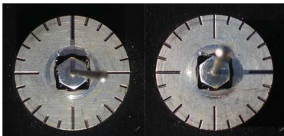
Fig. 19. The BioSCAN solar compass a ) pointed (down) into the sun plane (left), and b ) pointed (CW) perpendicular to the sun plane (right).
