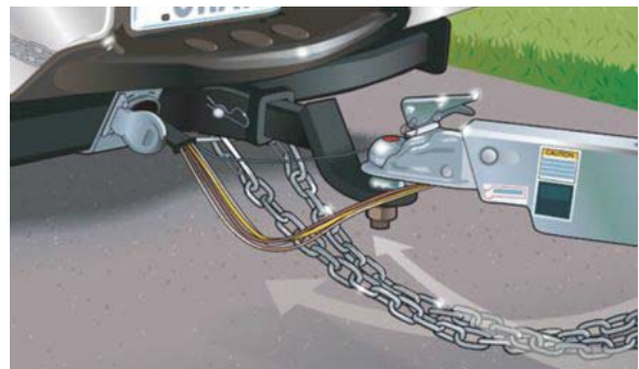
Fig. 37. A partial view of a trailer attached to a hitch, showing the coupler attached to the hitch ball on a receiver with crisscrossed safety chains attached below ( http://www.boat-ed.com ).
