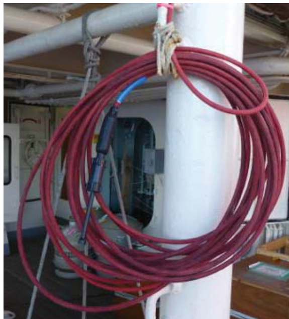
Fig. 15. An example of a cable extension that is disconnected and secured each day, so the cable bucket and C-OPS profiler can be stowed for safety.
