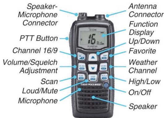
Fig. 18. An example R/T handset (model iM36, Icom Inc., Osaka, Japan) with antenna not attached and some important features labeled.
