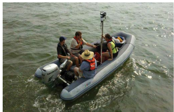
Fig. 39. The installation of a bar-stool mount for the C-OPS solar reference with BioSHADE and BioGPS on a small inflatable launched from the R/V SRV-X into the Blackwater National Wildlife Refuge.
