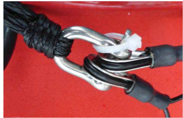
Fig. A6. A small cable tie fed through the shackle pin eye and looped around the shackle pin on the C-OPS harness to prevent the shackle from coming loose during deployments aboard the R/V Shearwater .
