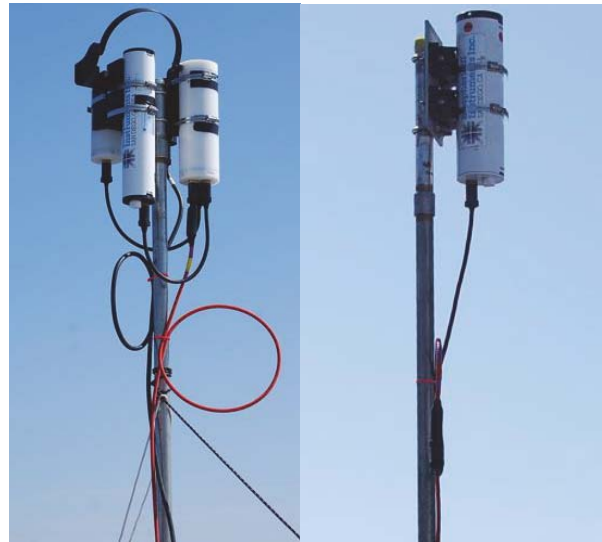
Fig. 12. Pipe masts on the R/V Gulf Challenger showing the following: a) the C-OPS reference plus BioSHADE and BioGPS accessories, with guy lines for stabilization and slack cable coils to facilitate sensor handling (left); and b) the older (and larger) SuBOPS reference mounted to a v-block on a flat plate (right), wherein the slack coil is perpendicular to the image and not easily discerned.
