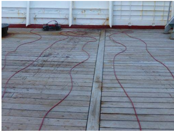
Fig. B9. The C-OPS instrument awaiting deployment (upper left) with the sea cable flaked onto the deck of the TR/V Oshoro Maru in the Bering Sea.
