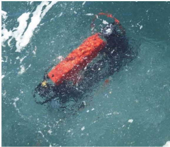
Fig. A5. The C-OPS backplane in the thruster turbulence of the TR/V Oshoro Maru revealing the large amount of small bubbles formed as a result of using the bow thruster.
