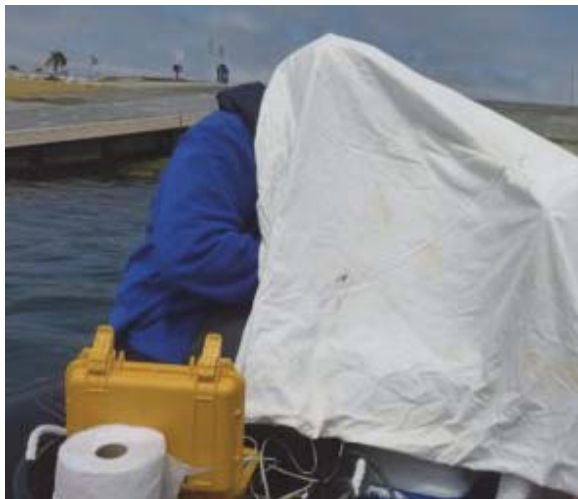
Fig. 40. Using the sheet that protects the profiler from overheating in sunshine as a shade, so the data acquisition computer screen can be seen in bright sunlight on board the R/V Recon 18 .
