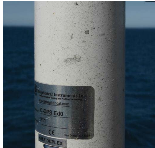
Fig. 31. The solar reference irradiance instrument after 10 dy at sea aboard the TR/V Oshoro Maru in the Bering and Chukchi Seas during which the ambient wind exceeded 20 kts ( 37 \text{ km hr}^{-1} ).
