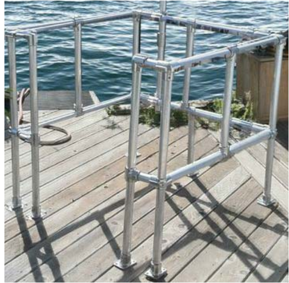
Fig. 14. A portable (all aluminum) open-rail platform for mounting the BioSCAN on the R/V Pelican while providing a secure area for the operator.
