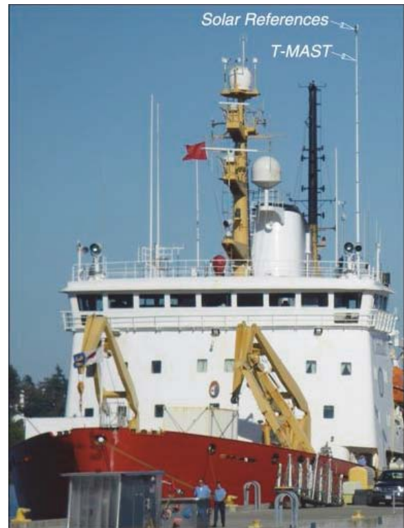
Fig. 29. A Telescoping Mount for Advanced Solar Technologies (T-MAST), the precursor device to BioMAST, aboard the CCGS Amundsen which, when deployed, placed the solar references at the highest point on the ship.
