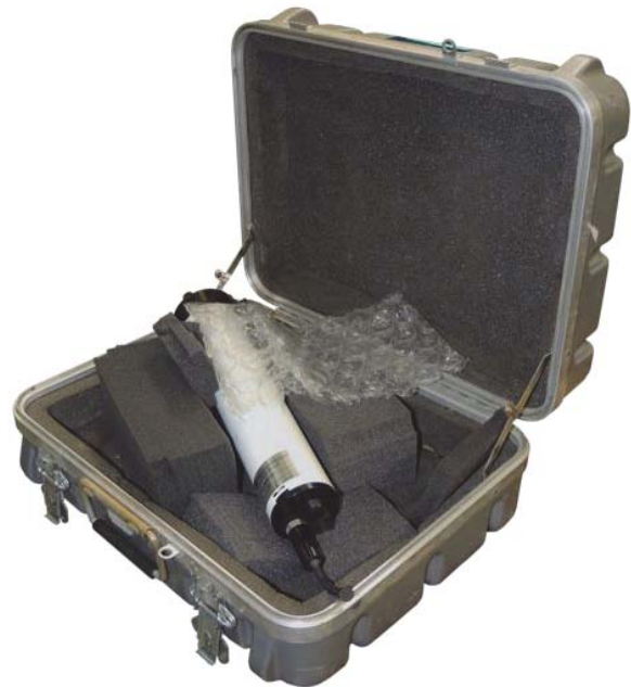
Fig. 35. An improperly packed instrument sent to the manufacturer wherein loose packing material permitted the instrument to tumble inside the container and completely flatten a piece of bubble wrap insulating material (courtesy J. Morrow).
