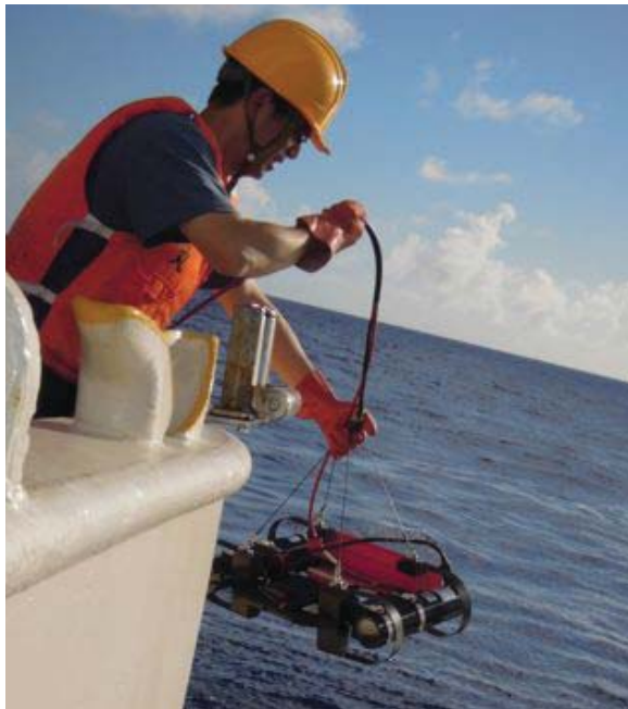
Fig. 23. Lowering the C-OPS over the side of the R/V Hakuho Maru with a hand-over-hand motion.
