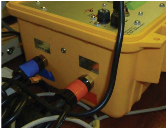
Fig. B3. Cable connections to the deck box with port 1 (underwater) labeled blue and port 2 (surface) labeled orange aboard the R/V Hakuho Maru .
