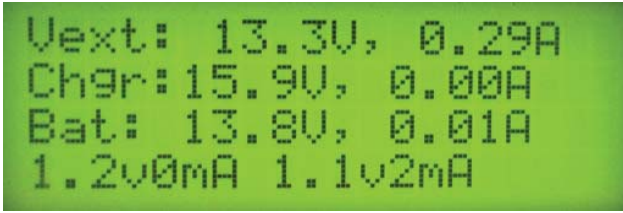
Fig. A4. A single deck box panel display during a normal power-up sequence as recorded with a digital camera aboard the R/V John Le Conte .
