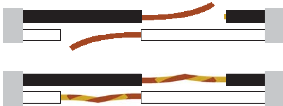
Fig. 34. A schematic of a staggered splice with the ground wire and heat-shrink tubing omitted for clarity: the wires stripped back within the gray over jacket and the bare conductors laid across one another at angles (top), so they can be twisted together and soldered (bottom).
