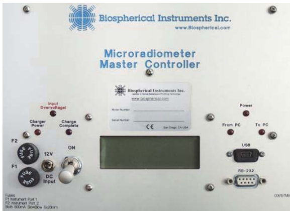
Fig. 8. The front panel of a BioSCAN or C-OPS deck box showing the power switch (slightly below and left of the green display) latched in the off position.
