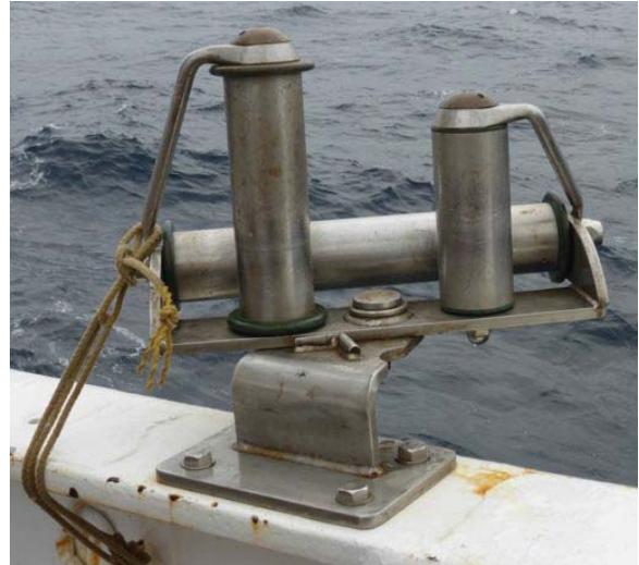
Fig. B4. A roller assembly to protect line or cable when hauled aboard the TR/V Oshoro Maru .
