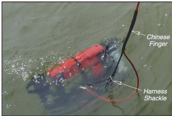
Fig. B7. The chinese finger on a C-OPS sea cable deployed from a small inflatable launched from the R/V SRV-X into the Chesapeake Bay.
