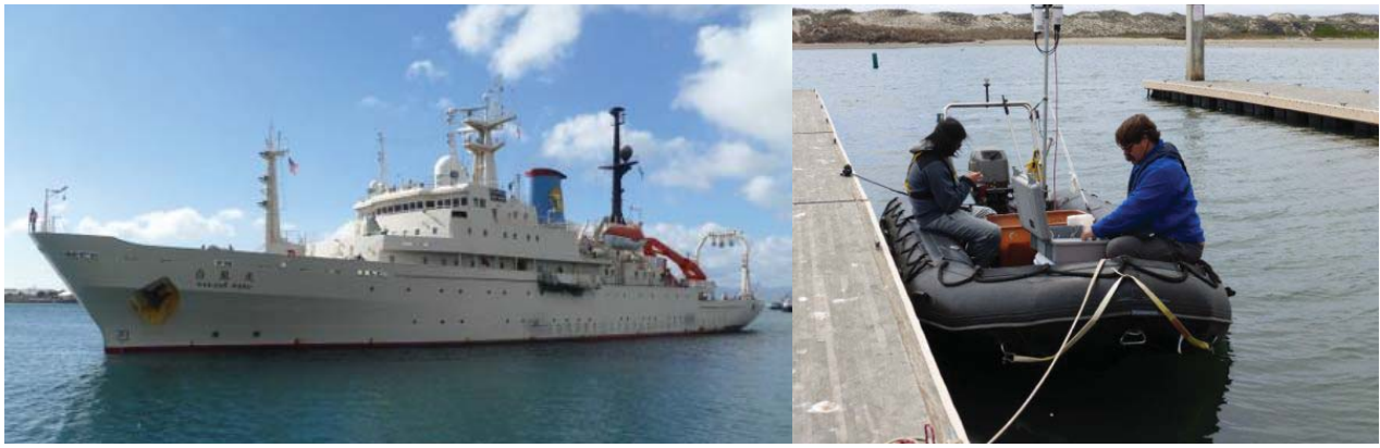
Fig. 2. The two end members in platform sizes showing a) the ocean-class R/V Hakuho Maru (left), with the height of a person standing on the bow setting the scale, and b) the small inflatable boat R/V Recon 18 (right). The former displaces almost 4,000 tons with an overall length of 100 m and two 1,085 kW generators developing 2,910 hp for propulsion, whereas the latter is a FC 470 military 4.7 m Zodiac fitted with a 30 hp Nissan outboard and custom-equipped for instrument deployments including 12 VDC and 120 VAC power.
