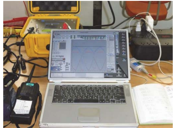
Fig. 9. An example acquisition computer environment aboard the TR/V Oshoro Maru showing the following: laptop computer (center foreground), marine radio (left of computer), written log (right of computer), C-OPS deck box (background left), and a small UPS (background right).
