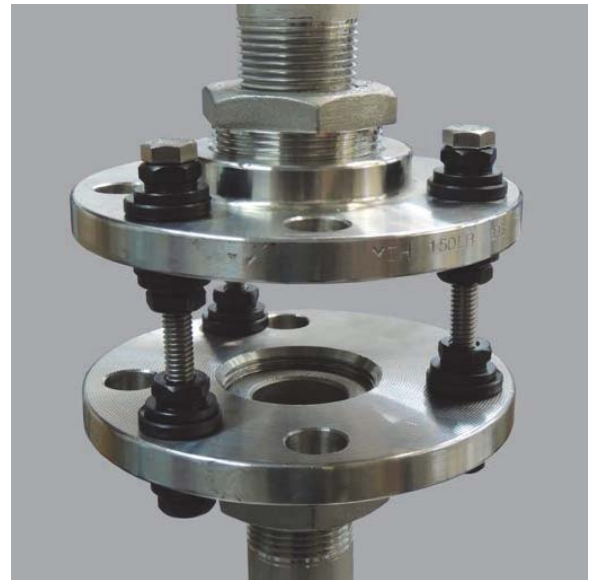
Fig. B12. The prototype BioFLAAT device built from two 1½ in 316SS pipe flanges. Black passivated components were used for simplicity and to improve clarity (courtesy J. Morrow).
