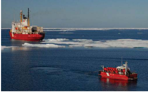
Fig. 36. The small boat or barge launched from the CCGS Amundsen wherein the smaller vessel could drift into sea ice areas with minimum mixing of the water mass to be sampled.
