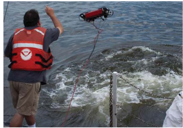
Fig. 24. Knifing the C-OPS backplane into the propeller turbulence aboard the R/V SRV-X in the Chesapeake Bay.
