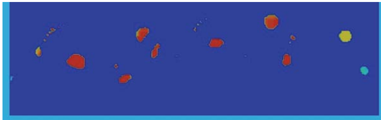
Figure 4. The vortex core radii at the grid points where the scaled Q-criterion is greater than or equal to 1.
