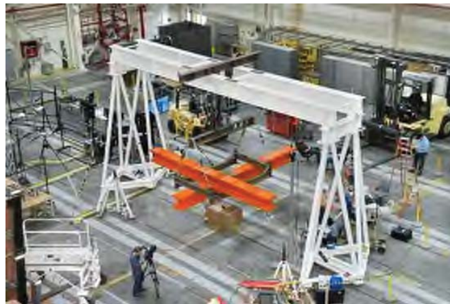
Figure 4. The iron bird undergoing I zz pendulum testing.
