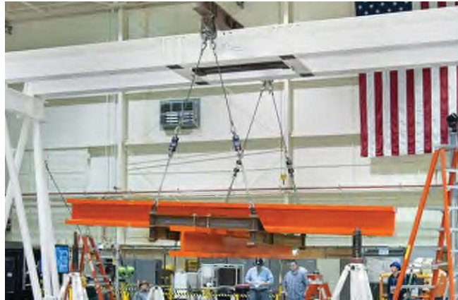
Figure 3. The iron bird undergoing I xx pendulum testing.
