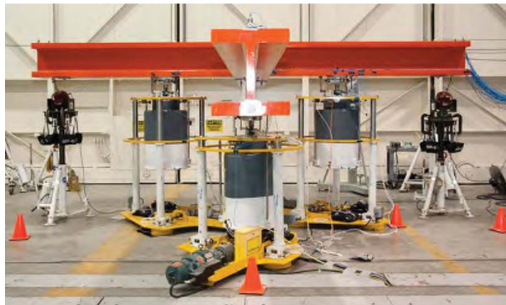
Figure 7. The iron bird undergoing DIM testing on soft supports.
