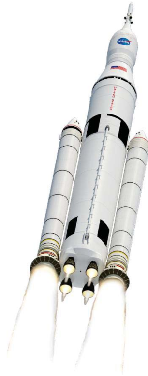
Figure 1. Space Launch System Block I Vehicle.
