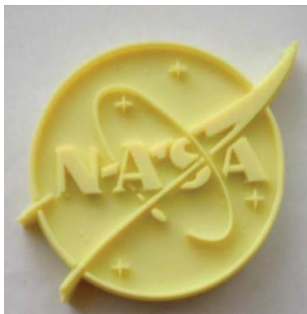
Figure 16. A OAPS cross-linked polyimide aerogel sample made with BPDA and DMBZ.
