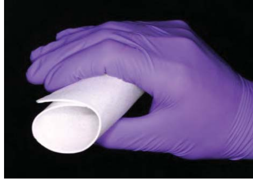
Figure 28. Aerogel composite reinforced with APA-2 paper.
