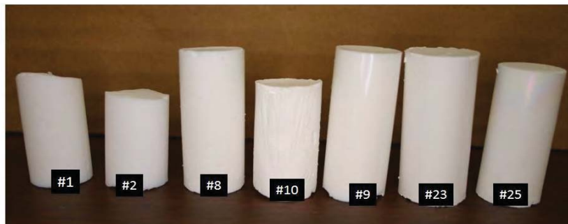
Figure 9. Photos of the selected samples made with BTSPD, TMOS, and VTMS. (Reproduced from Publication 24 with the permission from The Royal Society of Chemistry.)
