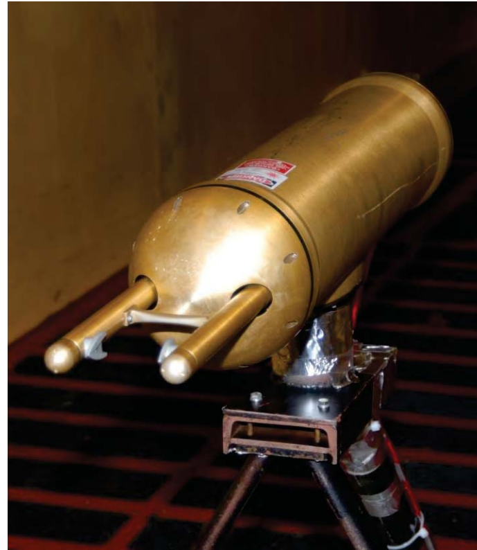
Optical Array Probe OAP-230X 15 – 450 \mu\text{m}
