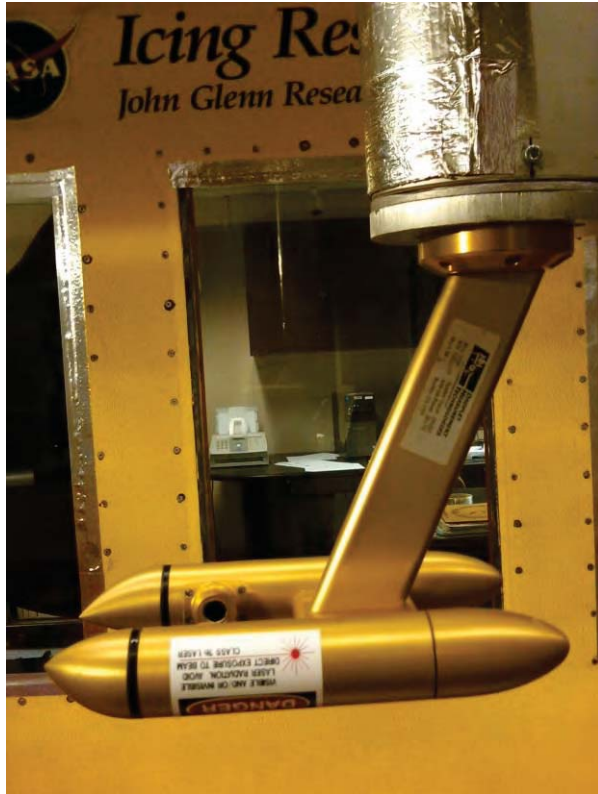
Cloud Droplet Probe CDP 2 – 50 \mu\text{m}
