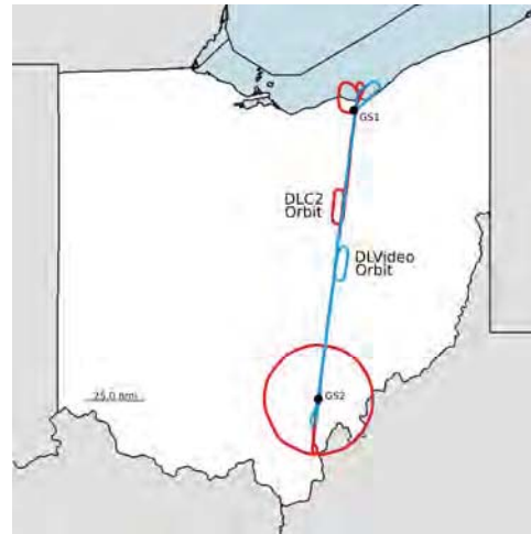
Figure 12. - Aircraft flight track for characterization of ground station 2. Flight track created using GPS Visualizer [8], Map data from the National Atlas [10]
