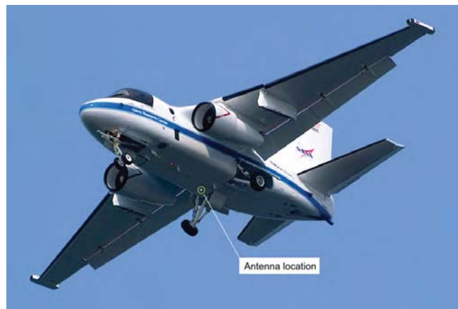
Figure 8. - S-3B Viking test aircraft showing L-band antenna mounting location. Image © 2008 – TarmacPhotos.com [9], used with permission
