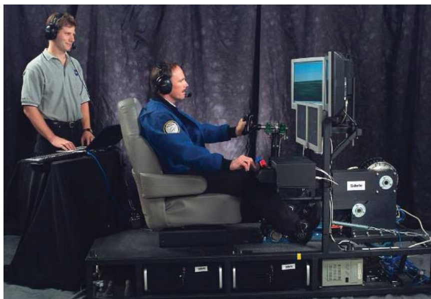
Figure 7.—NASA's Ice Contamination Effects Flight Training Device (ICEFTD)
